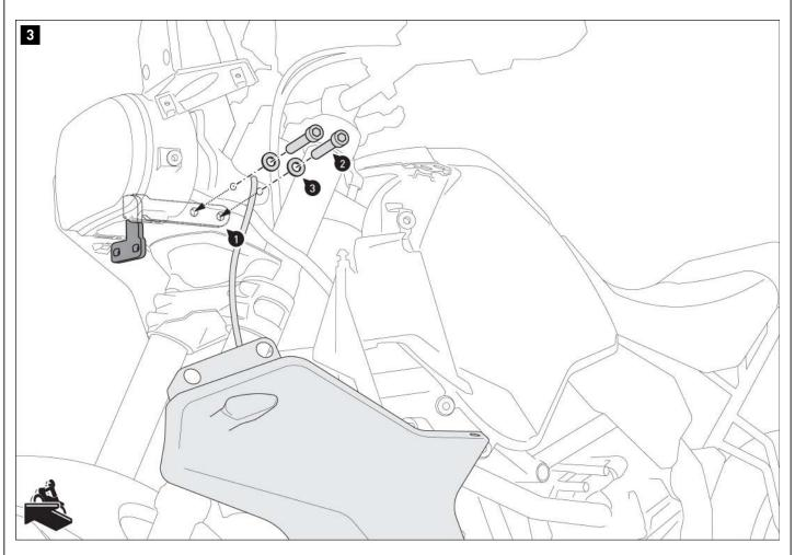
Screw the mounting bracket on the left side of the vehicle (1) to the inside of the steering head.
