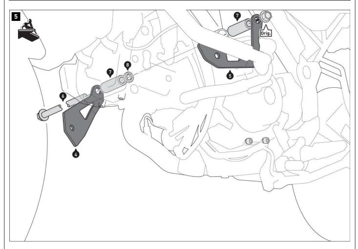
$\triangle$ **NOTE:**Use the indicated parts when mounting the SW-MOTECH crash bar at the same time. The crash bars are screwed onto the mounting brackets (4) and (5).
