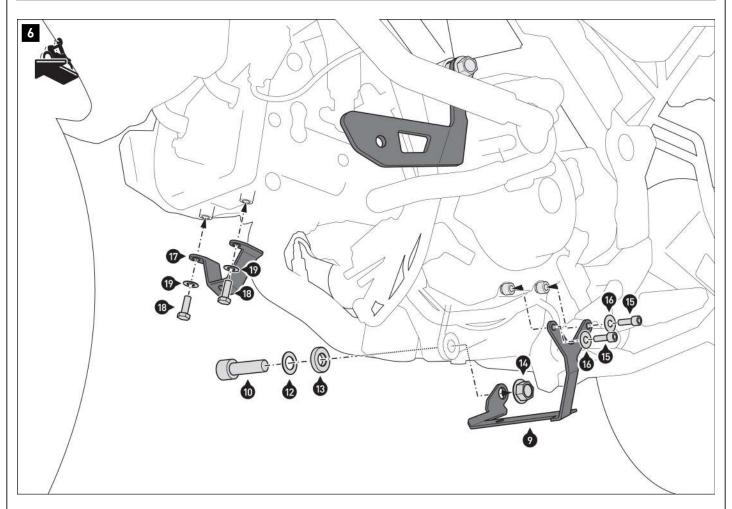
$\triangle$ **NOTE:** Use the screw (11) at the left attachment point when mounting the SW-MOTECH centerstand at the same time. Parts (12) and (13) are omitted. Use the parts on the centerstand instead.
