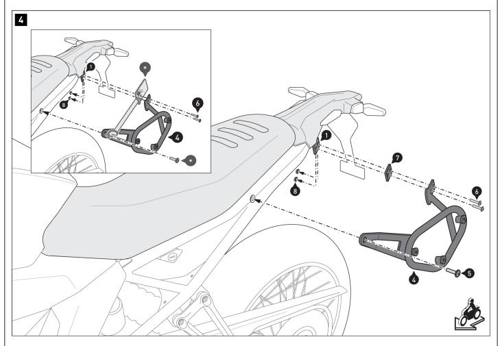
$\triangle$  **NOTE:** When installing at the same time as the SW-MOTECH rack (\*), screw the parts together as shown in the detailed drawing. The spacer (7) and screw (5) are no longer required. Instead, use the screw (\*) that comes with the carrier.
