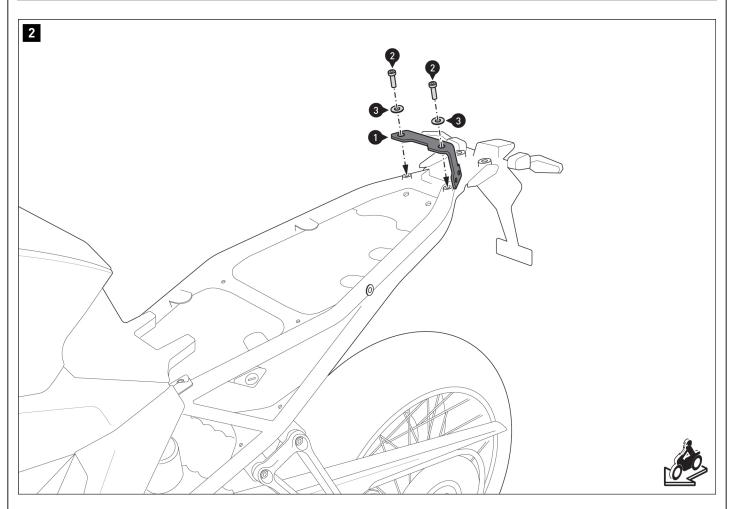
Screw the mounting bracket (1) onto the vehicle. **A** WARNING: Use liquid threadlocker!
