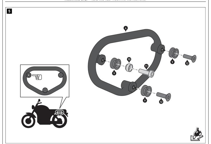
Screw the parts [9] to (12) onto the side carrier (4).
