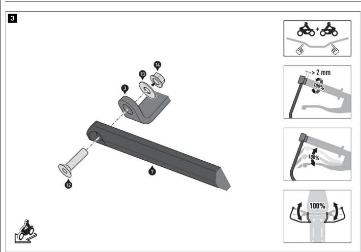
Screw the inner ends of the brackets (7/8) to the connecting plates (2/3). Do not tighten the screws (12) yet.
