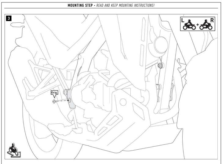
Screw the heel guards back onto the vehicle on both sides. Tighten the original (Orig.) screws according to the manufacturer's instructions.
