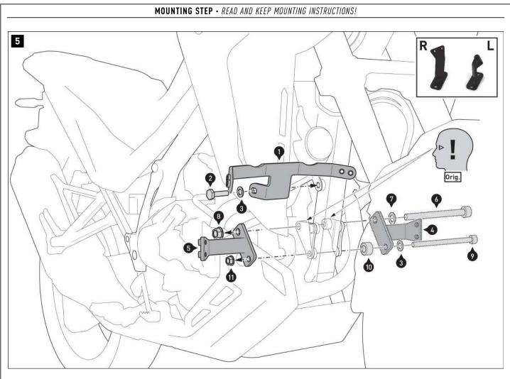
Mount the crossbar (1) and the mounting struts (4/5) on the vehicle frame. **A WARNING: Use liquid screw locker for screw (2).** Do not tighten the screws yet.
