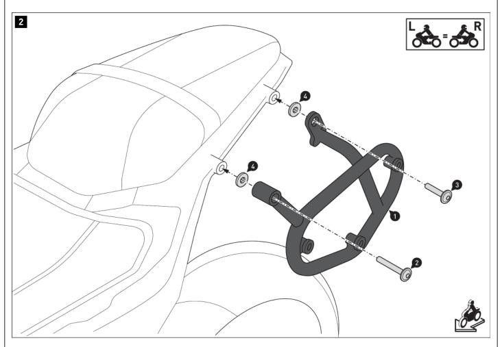
Screw the side carrier (1) to the rear of the vehicle.
