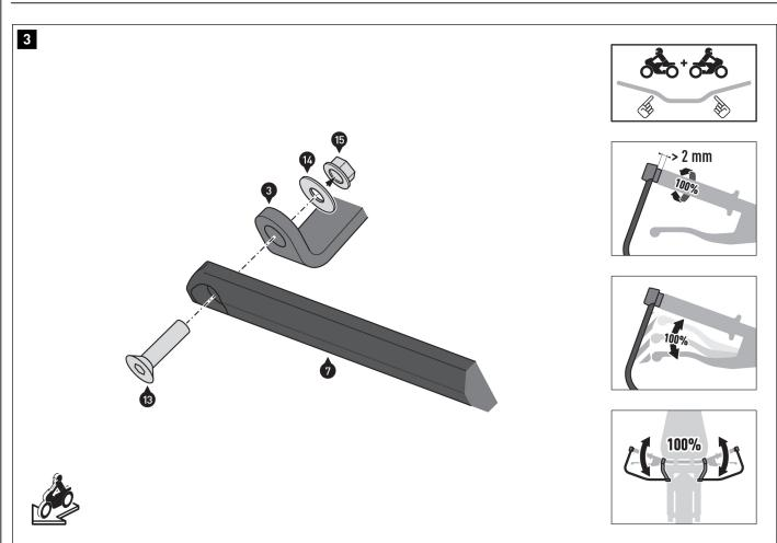
Screw the inner ends of the brackets (7/8) to the connecting plates (2/3). Do not tighten the screws (13) yet.
