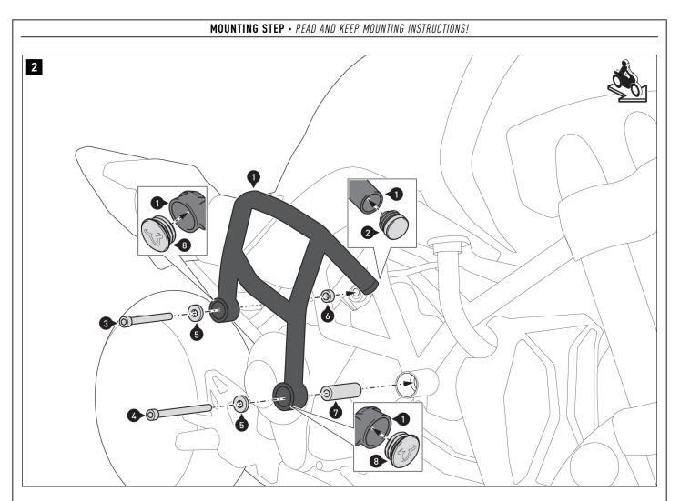
Insert the plastic plug (2) into the opening of the crash bar (1).
