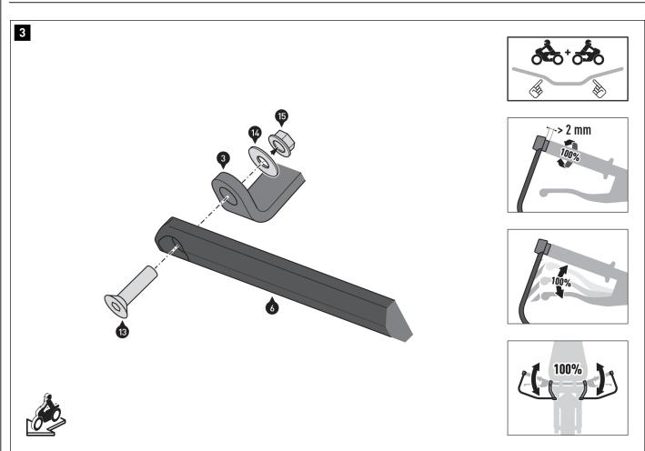
Screw the inner ends of the brackets (6/7) to the connecting plates (3/4). Do not tighten the screws (13) yet.
