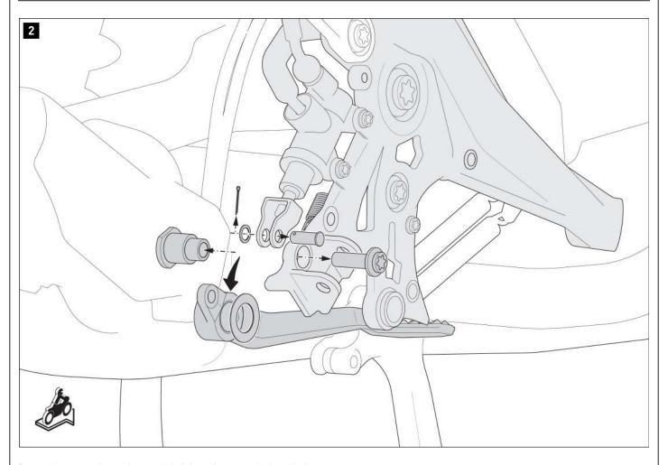
Remove the cotter pin, and loosen the bolt from the master brake cylinder. Loosen the original screws from the footrest mount. Release the springs from the brake lever. Then remove the original brake pedal from the footrest mount.
