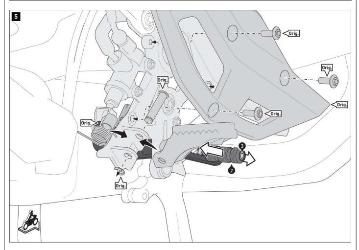
Attach the original footrest with the associated parts to the footrest mount. Screw the heel guard back onto the vehicle using the original screws (Orig.).
