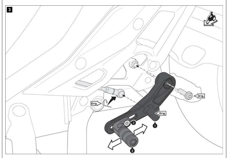
Insert the deflection rod onto the ball pin (Orig) screwed to the gear lever (1); secure the connection with the original safety bracket (Orig.).
