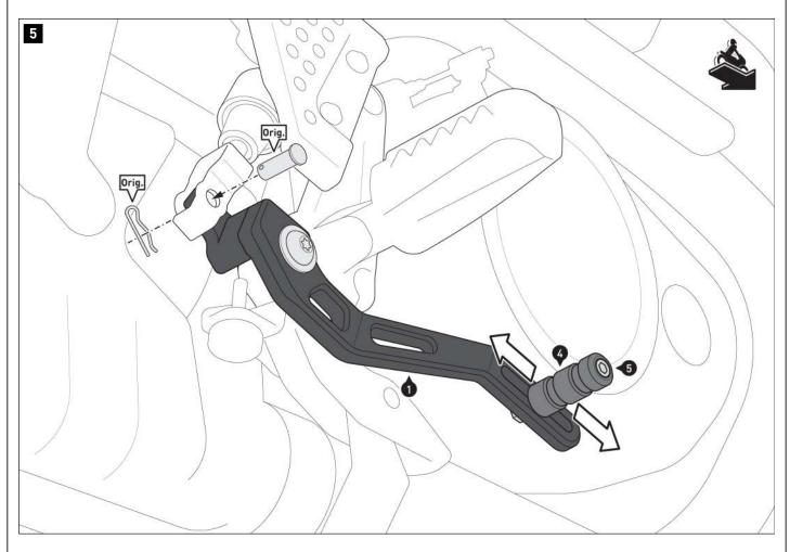
Connect the brake pedal (1) to the brake master cylinder. Use the original parts (Orig.).
