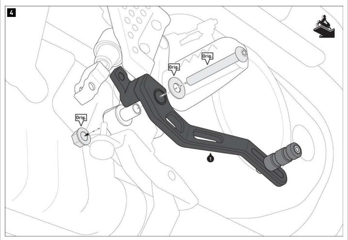
Screw the brake lever [1] to the vehicle using the original parts (Orig.). Tighten the original screw (Orig.) according to the manufacturer's instructions.
