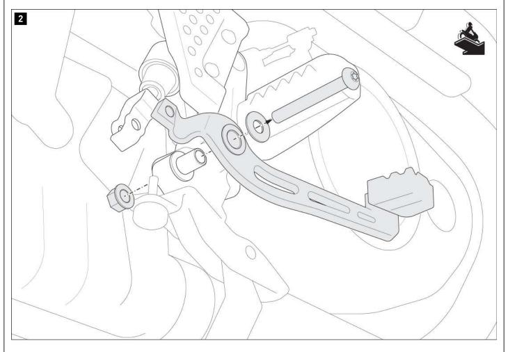
Remove the original brake pedal and the parts shown from the footrest mount.
