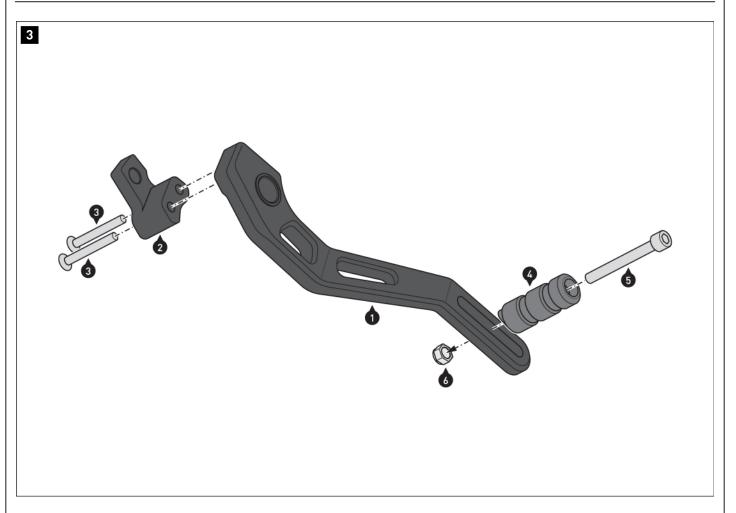
Screw the parts shown together. **A** WARNING: Use liquid thread locker (only the screws (3))!
