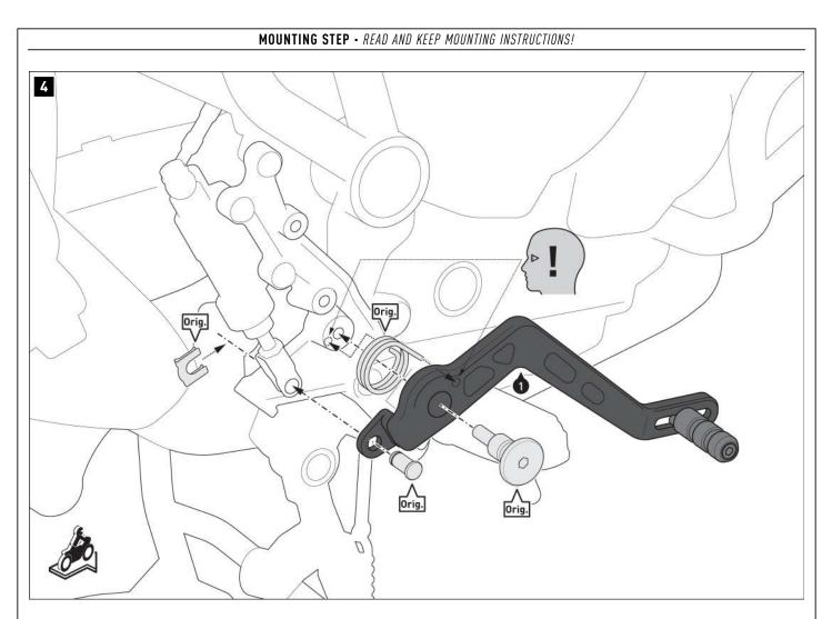
Screw the brake pedal (1) to the original parts (Orig.) screws. A WARNING: Be sure to insert the ends of the original spring (Orig.) into the holes provided! A WARNING: Use a liquid threadlocker! Tighten the original screw (Orig.) according to the manufacturer's instructions.
