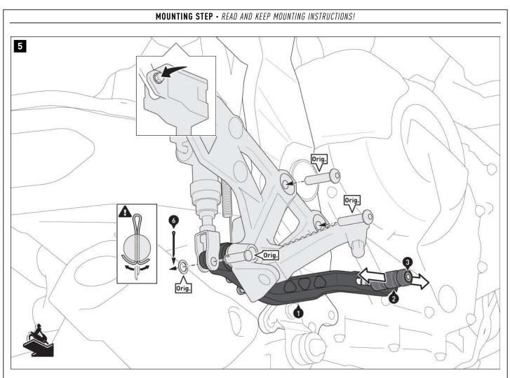
Connect the brake pedal (1) to the brake master cylinder. Use the original parts (Orig.). Secure the original bolt (Orig.) with the enclosed cotter pin (6).
