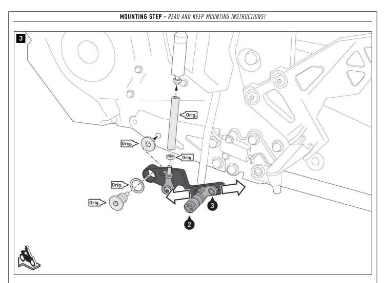
Screw the original deflection rod (Orig.) to the gear lever (1) (min. 6 threads); lock the thread with the two original nuts (Orig).
