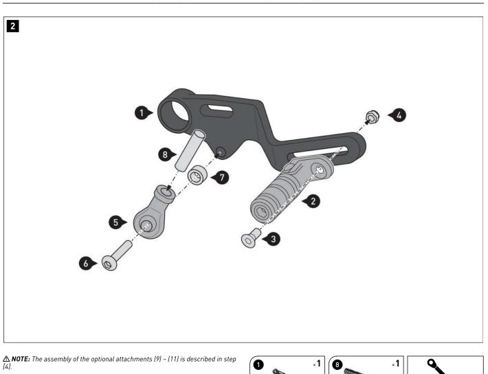
Screw the parts shown to the gear lever (1). **A WARNING: Use liquid thread locker (only for screw (6))!** Tighten the screw (6) as specified in the mounting instructions. Do not tighten the screw (3) yet.
