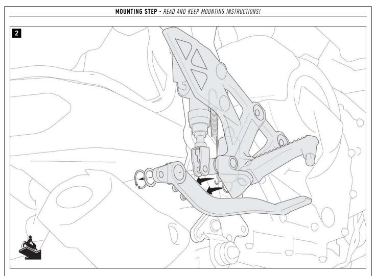
Release the springs from the brake lever. Then remove the original brake lever and the parts shown from the footrest mount.
