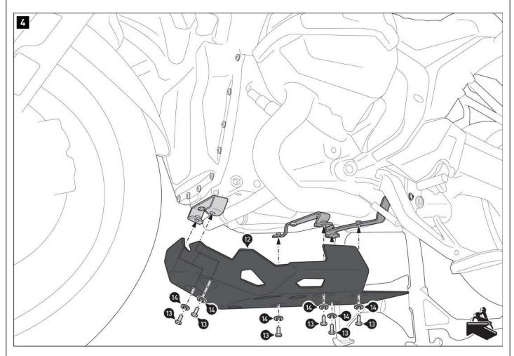
Screw on the engine guard [12]. **A WARNING: Use liquid thread locker!**Tighten the screws [13] as specified in the mounting instructions.
