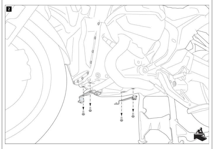
Remove the original retaining plates from the vehicle.
