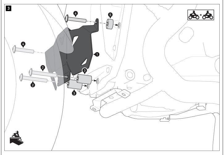
Screw the engine guard extension [1] onto the vehicle.
