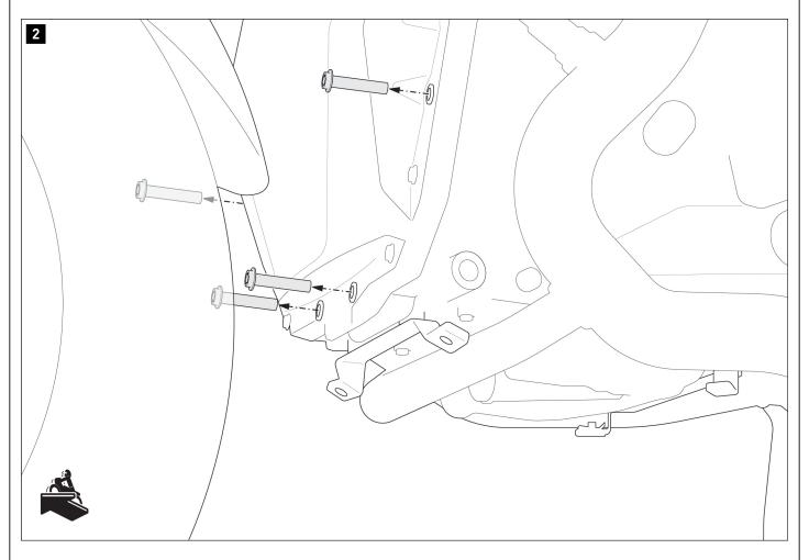
Remove the four original screws shown from the vehicle.
