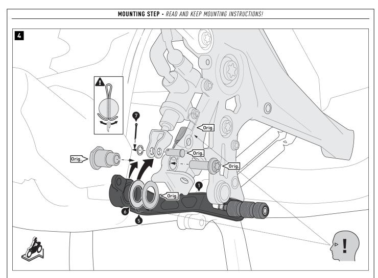
Screw the brake lever to the vehicle using the original parts (Orig.). A WARNING: Make sure to hook the end of the original spring (Orig.) onto the cradle suspension (5)!
