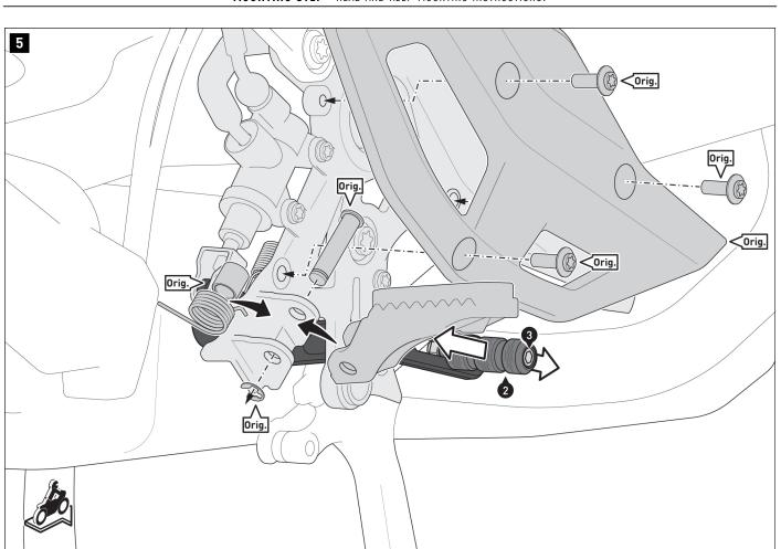
Attach the original footrest with the associated parts to the footrest mount. Screw the heel guard back onto the vehicle using the original screws (Orig.). **A WARNING: Use a liquid threadlocker!** Tighten the screws (Orig.) according to the manufacturer's instructions.
