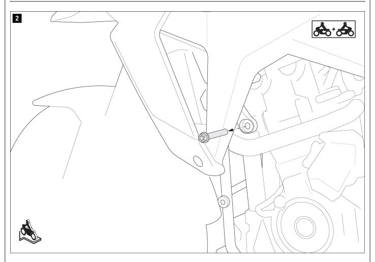
Push the side panel a little to the side to be able to remove the original screw.
