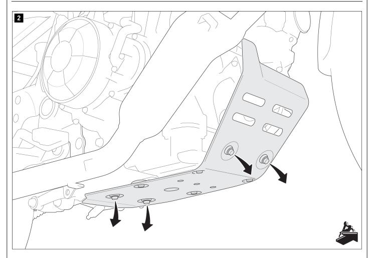
Loosen the four engine guard screws, and remove the engine guard from the vehicle.
