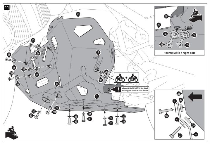
Screw the engine guard [28] onto the mounting supports, mounting brackets, and the front mounting points.
