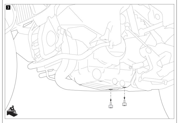
Remove the original rubber dampers shown.
