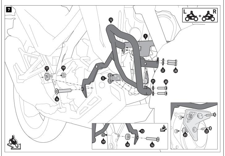
Screw the crash bars (12/13) to the vehicle, the crossbar (1), and the mounting struts (4/5).
