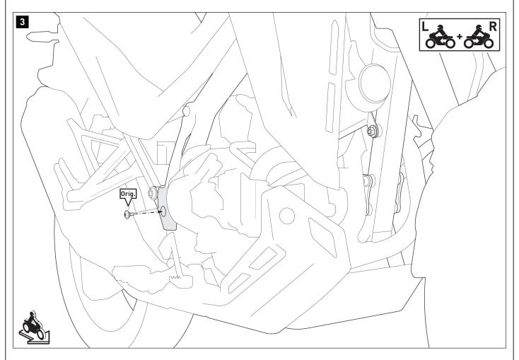
Screw the heel guards back onto the vehicle on both sides. Tighten the original (Orig.) screws according to the manufacturer's instructions.
