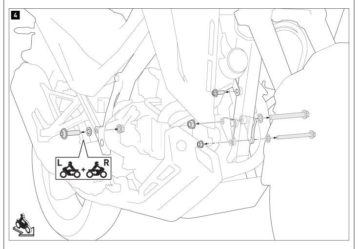
Remove the original screws, washers, and nuts (see drawing) on both sides of the vehicle.
