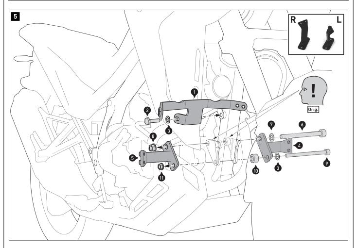
Mount the crossbar [1] and the mounting struts [4/5] on the vehicle frame.  $\triangle$  WARNING: Use liquid screw locker for screw [2]. Do not tighten the screws yet.
