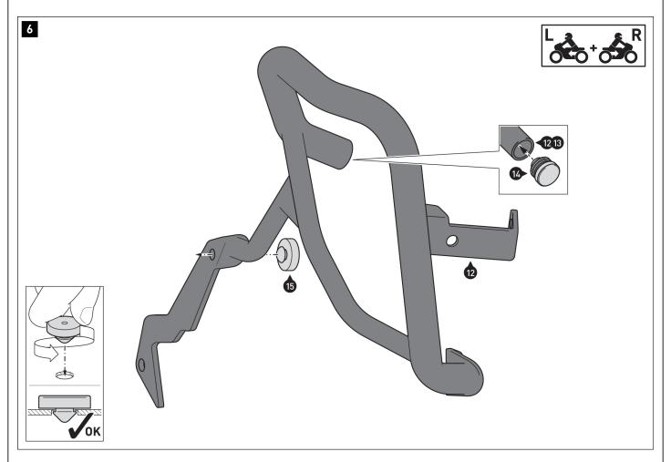
Insert the plastic plugs (14) and rubber dampers (15) into the crash bars (12/13).
