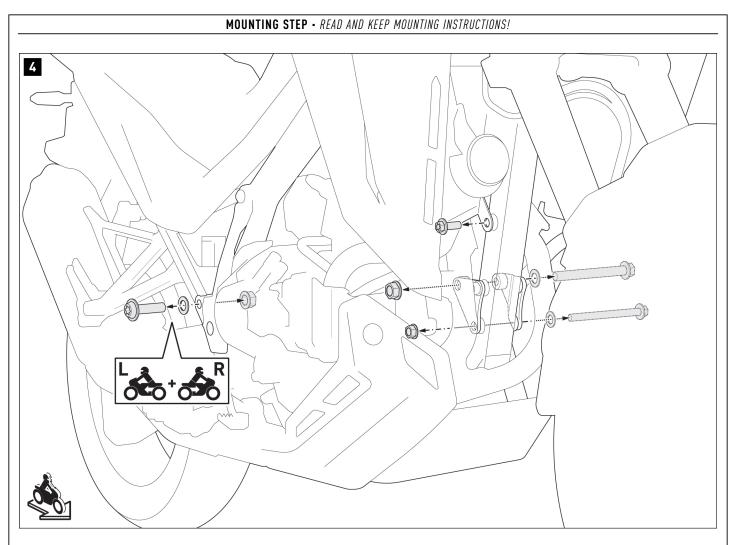
Remove the original screws, washers, and nuts (see drawing) on both sides of the vehicle. **MOTE:** Make sure to keep the original spacer shown (Orig.) in position.
