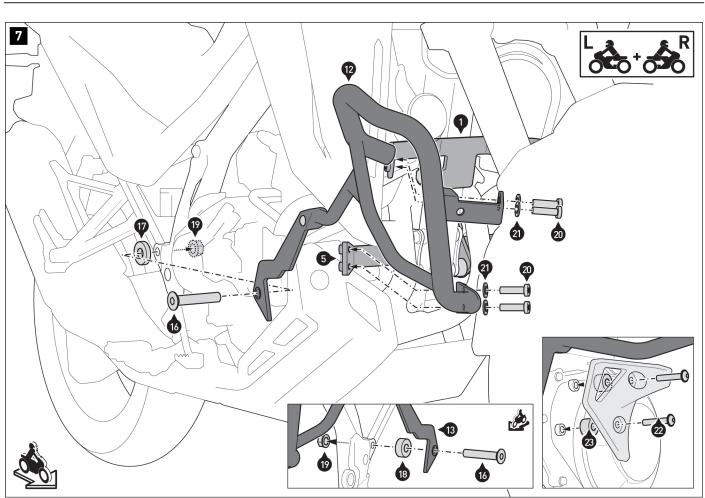
Screw the crash bars (12/13) to the vehicle, the crossbar (1), and the mounting struts (4/5). **A WARNING: Use Liquid screw locker for screws (20) and (22).** When all components are seated without tension, tighten the screws in the following order: (6), (9), (20), (2), (16), (22). Tighten the screws (22) according to the manufacturer's instructions. Tighten all remaining screws as specified in the mounting instructions.
