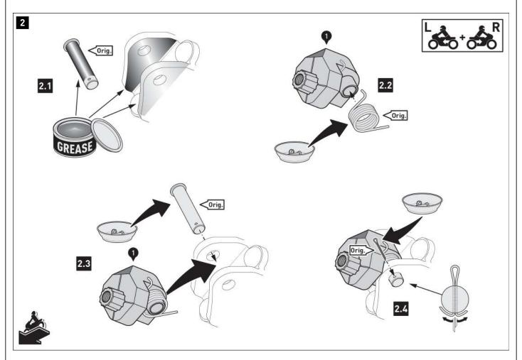
**Step [2.1]**: Clean the footrest mounts thoroughly. Apply some grease to the inside of the footrest mounts and the original bolts (Orig.).
