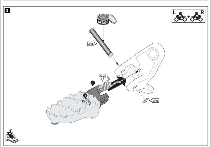
Clean the footrest mounts thoroughly. Apply rolling bearing grease to the (Orig.) bolts.
