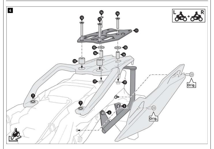
Screw the adapter plate [11] to the original rack.
