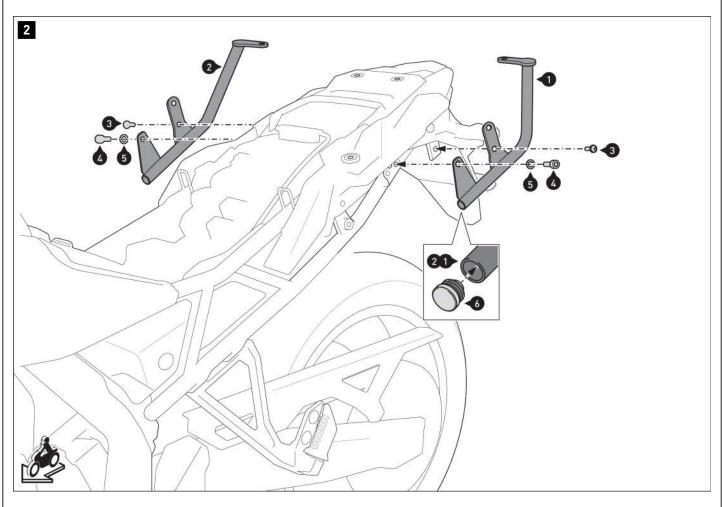
Insert the plastic plugs (6) into the openings on both sides of the side carrier.
