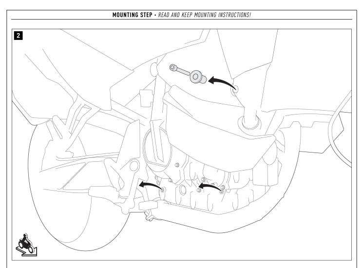
On the right side of the vehicle, remove the screws from the mounting points shown.
