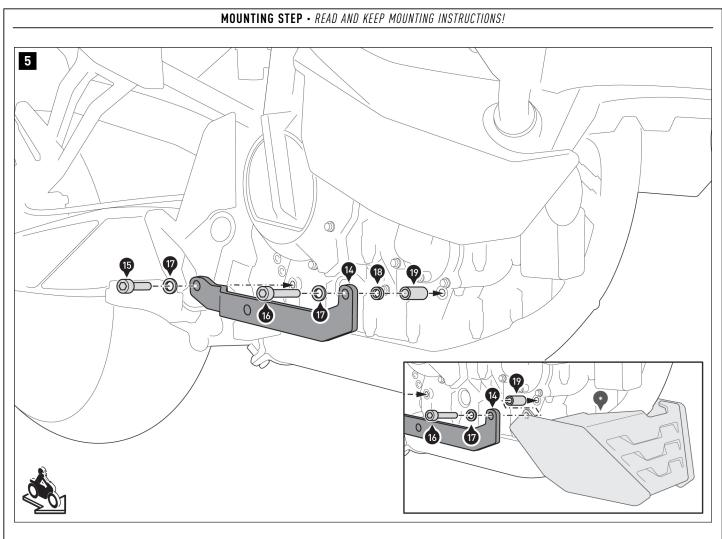
Screw the mounting bracket [14] onto the right side of the vehicle. **A WARNING: Use liquid threadlocker!** Do not tighten the screws yet.
