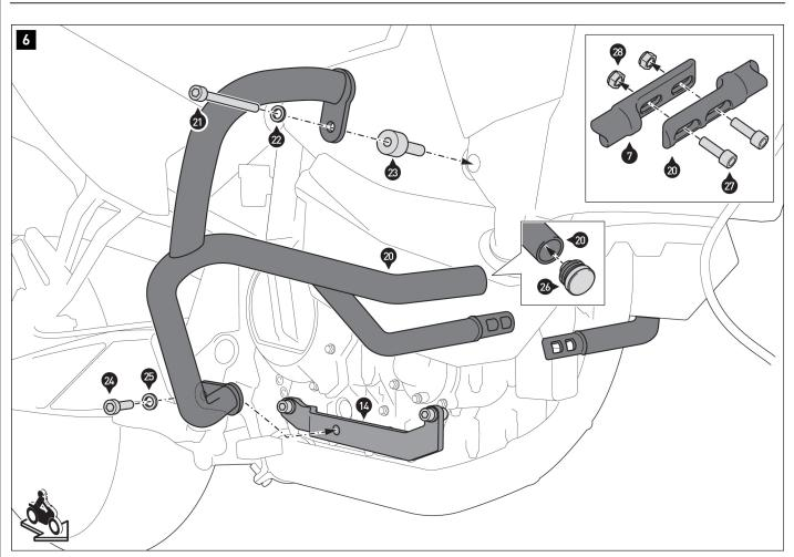
Insert the plastic plug [26] into the right half of the crash bar (20).
