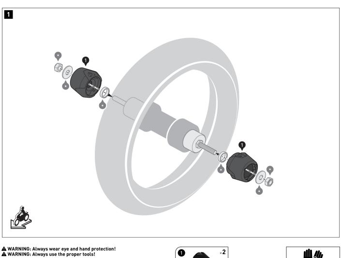
Assemble the crash pads (1) using the parts (\*) included in the crash pad kit. Tighten the nuts (\*) as specified in the frame slider kit mounting instructions.
