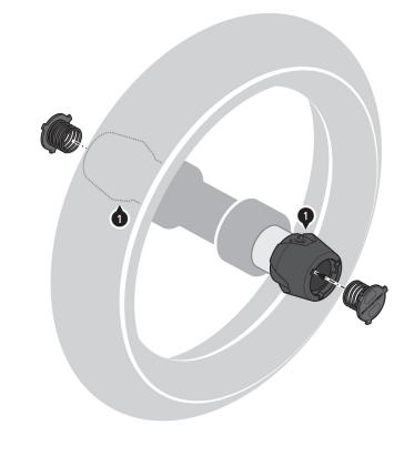
Insert the cover caps (2) into the openings of the mounted crash pads (1) on both sides and turn them to the end position. **NOTE:** Make sure that the cover caps (2) are firmly secured.
