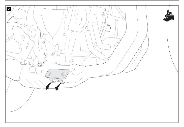
Loosen the indicated screws and remove the heat guard from the vehicle.
