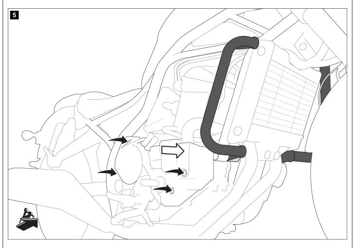
Screw the clutch cover back onto the vehicle. Tighten the screws according to the manufacturer's instructions.
