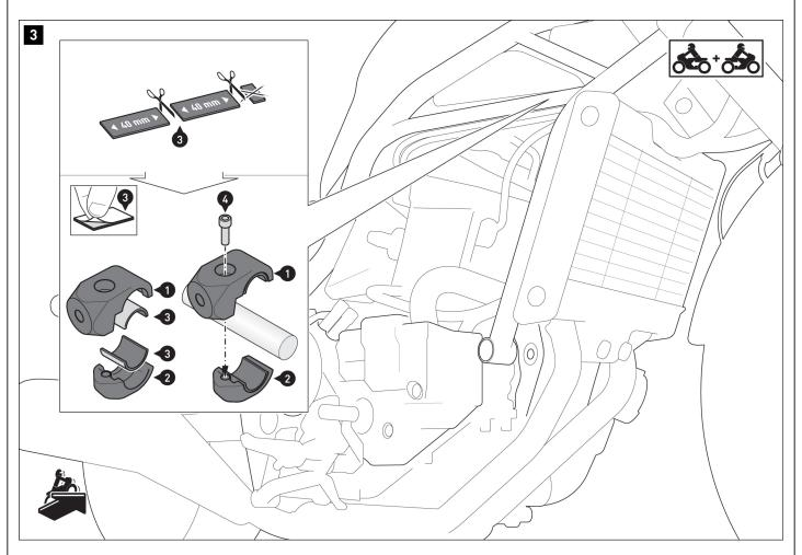
Cut each of the rubber strips (3) into two 40 mm pieces (the rest is no longer required).
