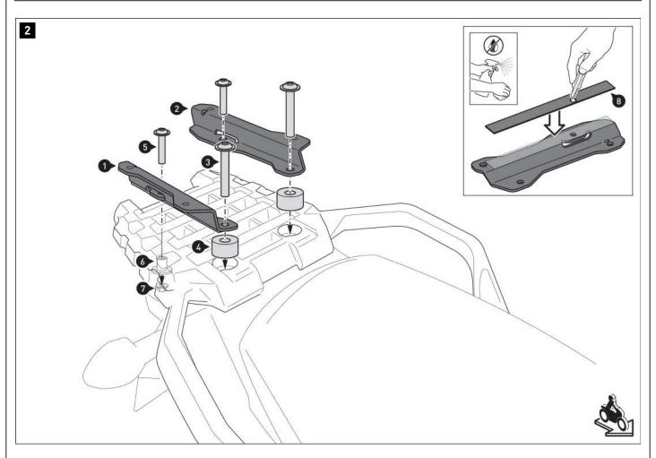
Clean the surface of the mounting brackets (1) and (2) and glue the protective strips (8) to their underside as shown in the detailed drawing. Cut openings for the now covered holes in the protective strips (8).
