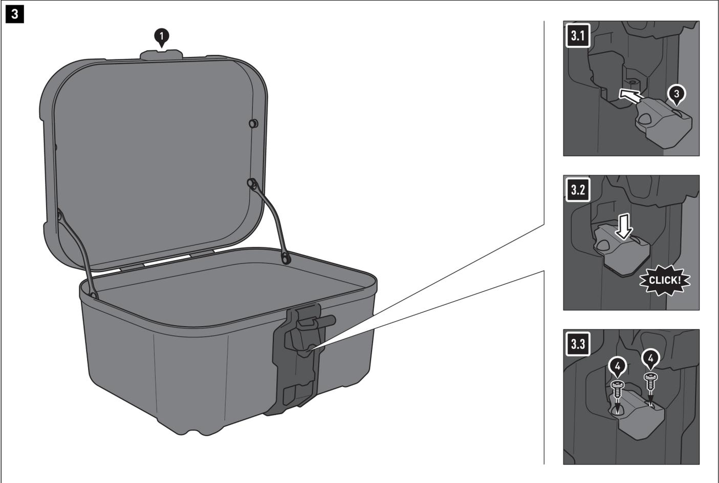
**Installing lock casing connector**
