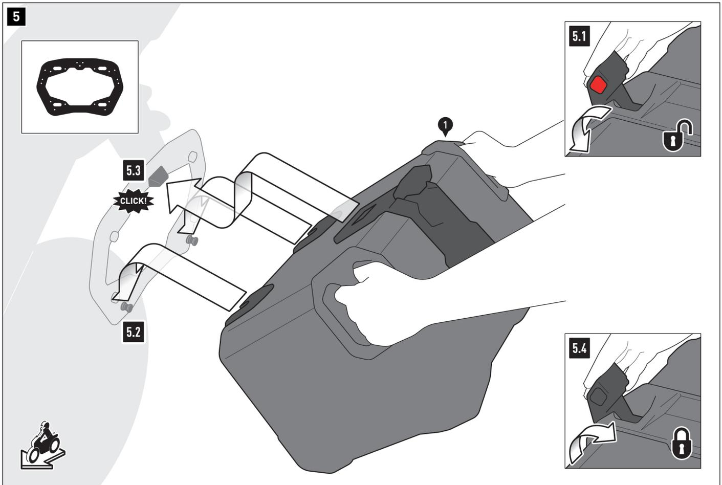
**Attaching the DUSC to a side case**
