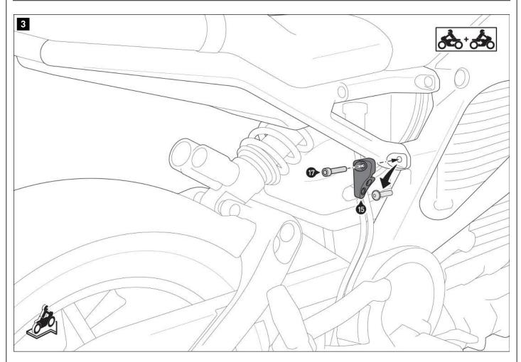
Loosen the original screws shown on both sides.
