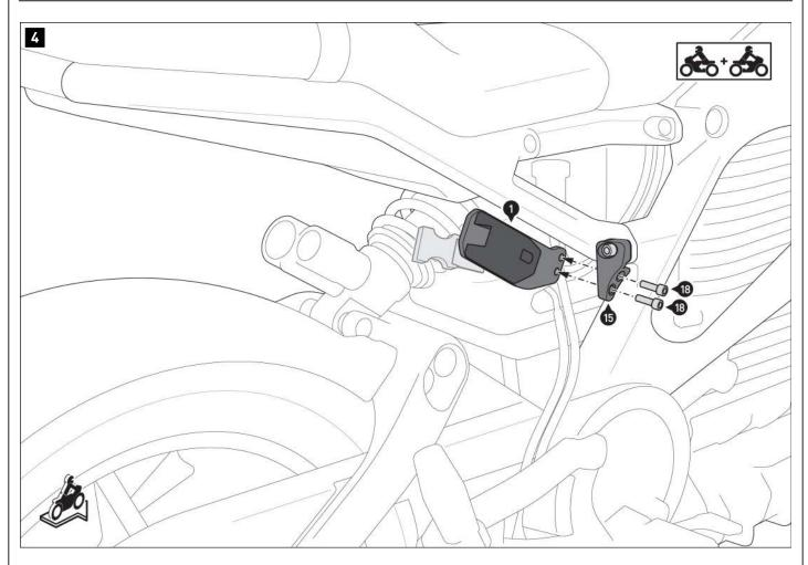
Screw the mounting brackets [1] / [2] to the milled parts [15] / [16]. **A WARNING:** Use a liquid threadlocker! Tighten the screws [18] as specified in the mounting instructions.
