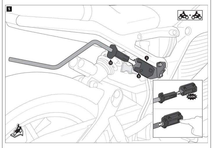
Insert the connectors (11) / (12) into the sockets (3) on both sides.
