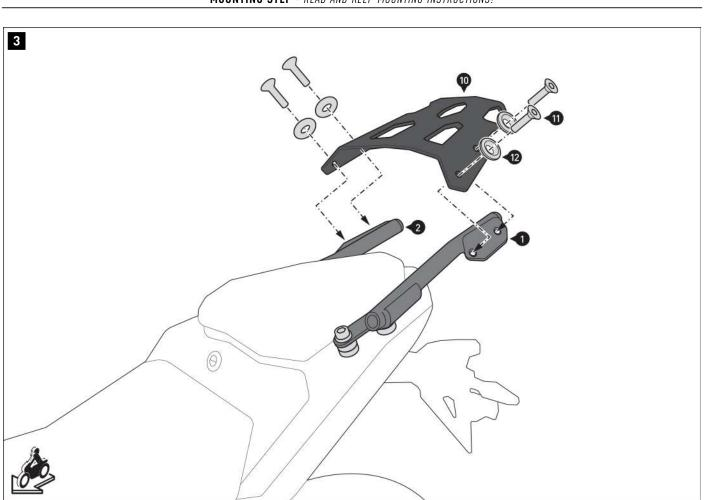
Screw the rack (10) onto the mounting struts (1) and (2). **A** WARNING: Use a liquid threadlocker!
