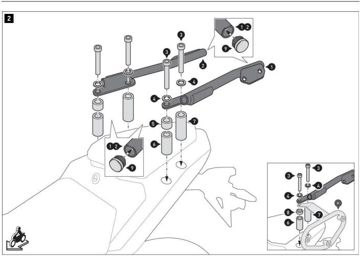
Insert the plastic plugs (9) into the ends of mounting struts (1) and (2).
