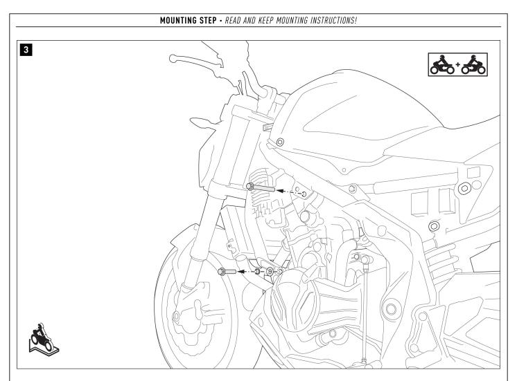
Remove the parts indicated from the vehicle.
