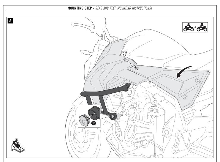
Install the side panel on the vehicle using the original screw (Orig.). **A WARNING: use liquid thread locker!** Tighten the original screw (Orig.) according to the manufacturer's instructions.
