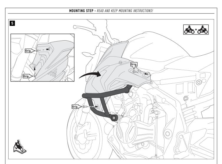
Install the side panel on the vehicle using the original screws (Orig.). **WARNING: use liquid thread locker!** Tighten the original (Orig.) screws according to the manufacturer's instructions.
