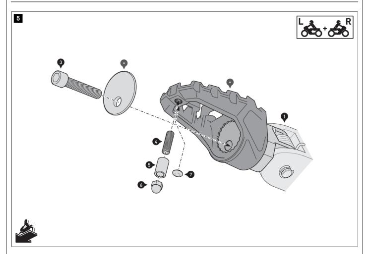
First screw the EVO footrest (\*) LOOSELY to the joint adapter (1/2). Check again for side-synchronous alignment and ergonomics.
