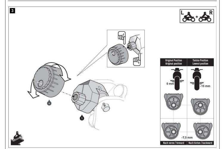
Insert the positioning cones (\*) onto the star-shaped receptacle cones of the joint adapters (1/2).
