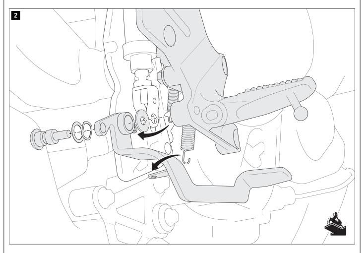
Release the springs from the brake lever. Then remove the original brake lever and the parts shown from the footrest mount.  $\frac{1}{2} \int_{\mathbb{R}^{n}} \frac{1}{2} \int_{\mathbb{R}^{n}} \frac{1}{2}$
