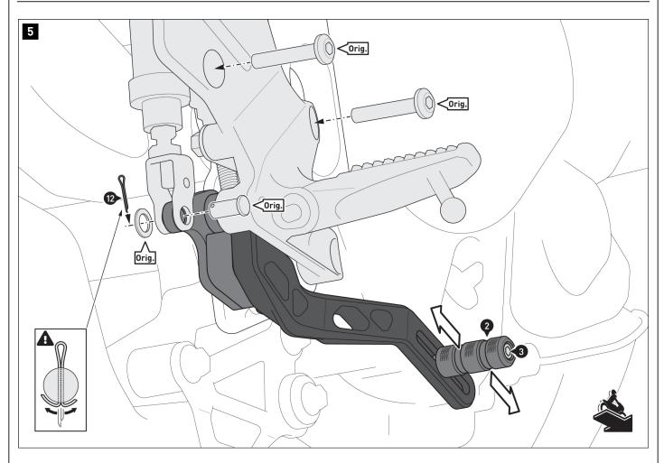
Connect the brake pedal (1) to the brake master cylinder. Use the original parts (Orig.). Secure the original bolt (Orig.) with the enclosed cotter pin (12).
