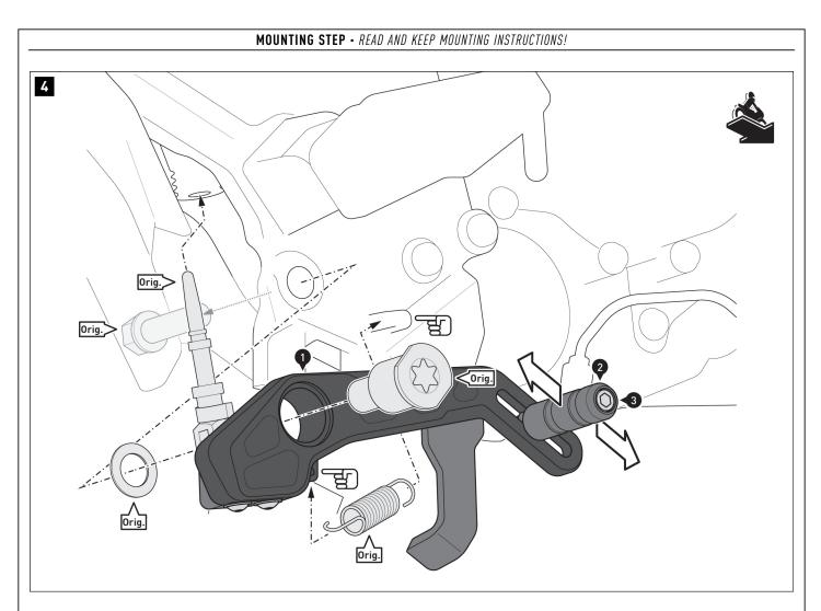
Insert the original pressure rod (Orig.) into the master brake cylinder.
