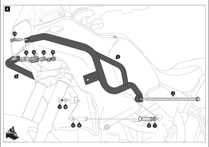
$\triangle$ **NOTE:** If the crash bars are fitted at the same time as the SW-MOTECH engine guard, spacers (7) and (9) are not required.
