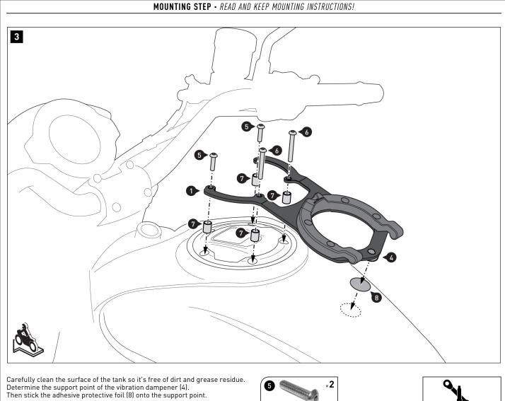
Screw the mounting bracket (1) to the vehicle. **A WARNING: Use a liquid threadlocker!** Tighten the screws according to the manufacturer's instructions.
