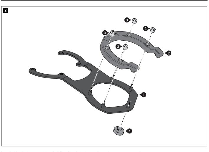
Insert the vibration dampeners (4) into the indicated opening in the mounting bracket (1). Carefully screw the tank ring (2) to the mounting bracket (1). Tightening the sleeve nuts (3) too tightly can damage the tank ring. **AWARNING: Use a liquid threadlocker!** Tighten the sleeve nuts (3) as specified in the mounting instructions.
