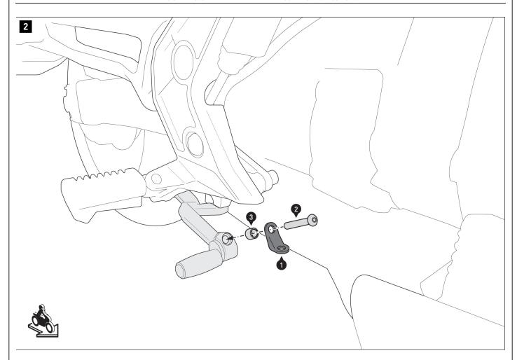
Screw the mounting bracket (1) to the brake pedal. **A WARNING:** Use a liquid threadlocker!
