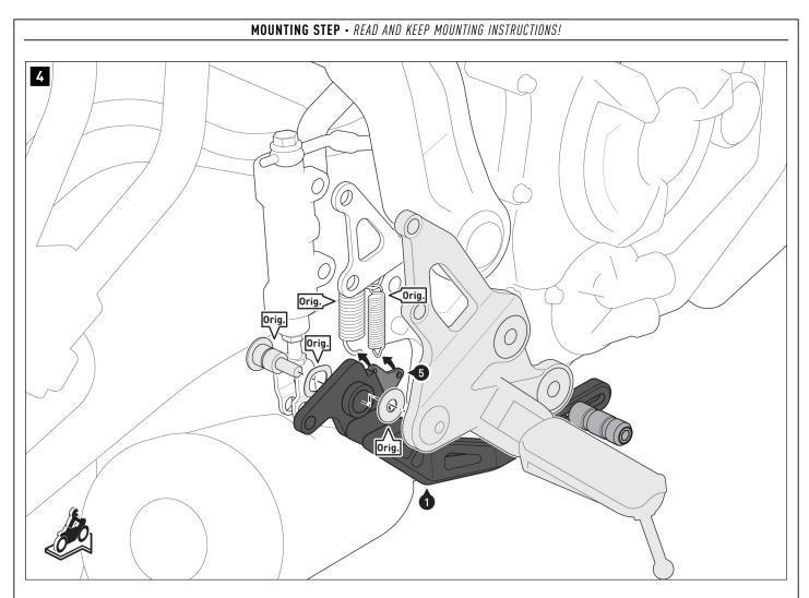
Screw the brake pedal (1) to the original parts (Orig.) to the footrest mount. A WARNING: Be sure to insert the ends of the original springs (Orig.) into the specially designed holes located on the spring bracket (5)! A WARNING: Use a liquid threadlocker! Tighten the original screw (Orig.) according to the manufacturer's instructions.
