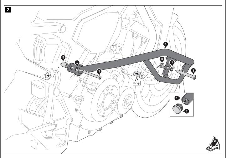
Insert the plastic plug (2) into the crash bar (1).
