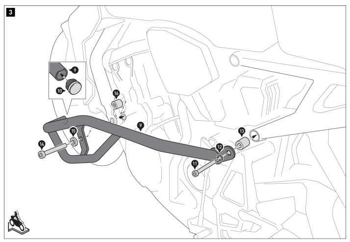
Remove the screws and spacer shown in step [1] on the left side of the  $\,$
