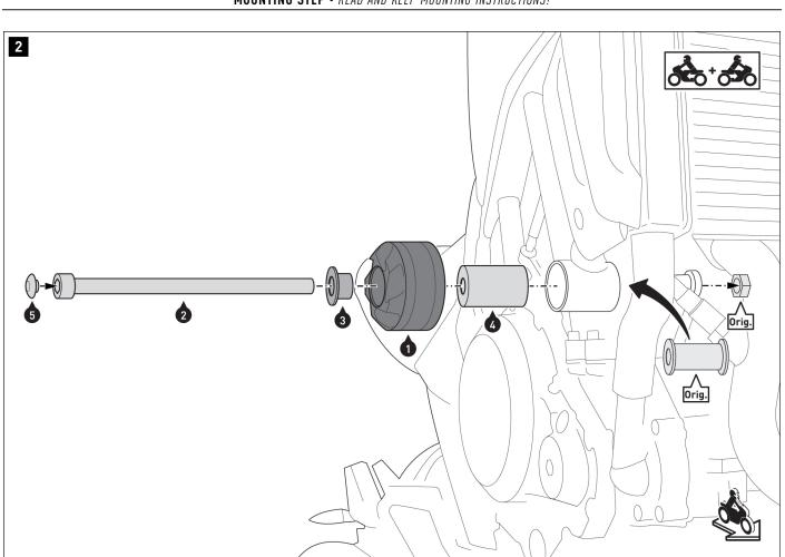
Screw the crash pad (1) to the vehicle using the original parts (Orig.) indicated. **A WARNING: Use a liquid threadlocker!** Tighten the screw (2) according to the manufacturer's instructions.
