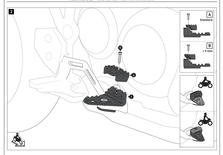
Screw the riser (45) onto the extension (1) in position [A] (standard) or [B] (+ 5mml.
