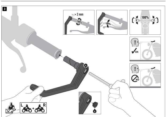
Insert the clamping bushes on the lever guards into the open handlebar ends on both sides up to the collar.
