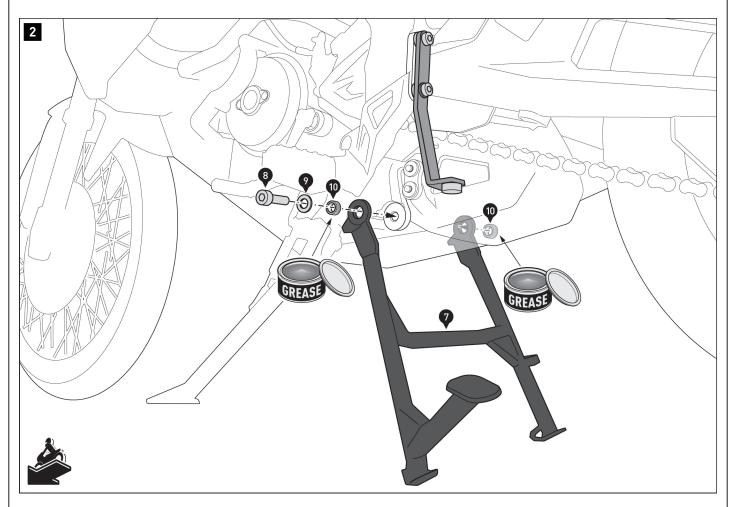
Coat the outside of the bearing bushings (10) with grease. Then insert the bearing bushings (10) into the openings on the centerstand (7).
