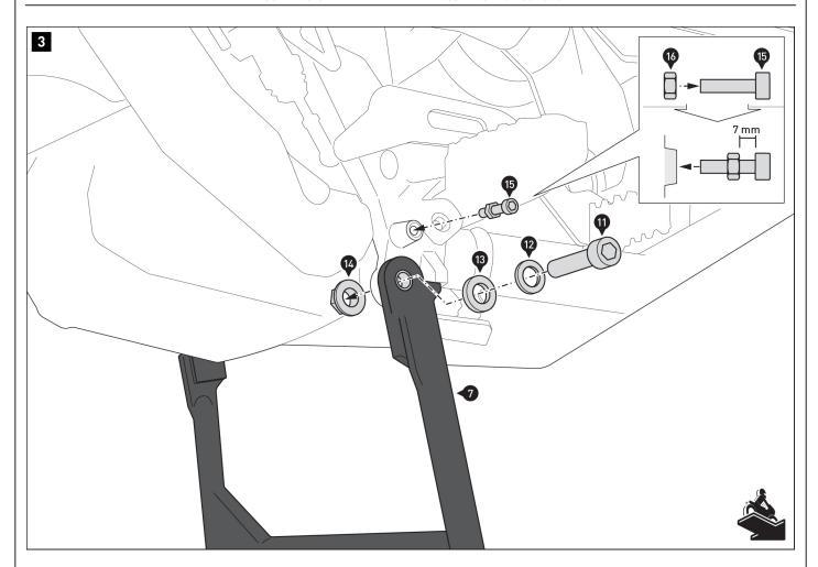
Screw the centerstand (7) onto the right-hand side of the vehicle. Now tighten the screws (8) and (11) according to the manufacturer's instructions.
