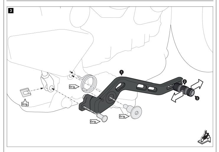
Screw the brake pedal (1) to the original parts (Orig.) screws.
