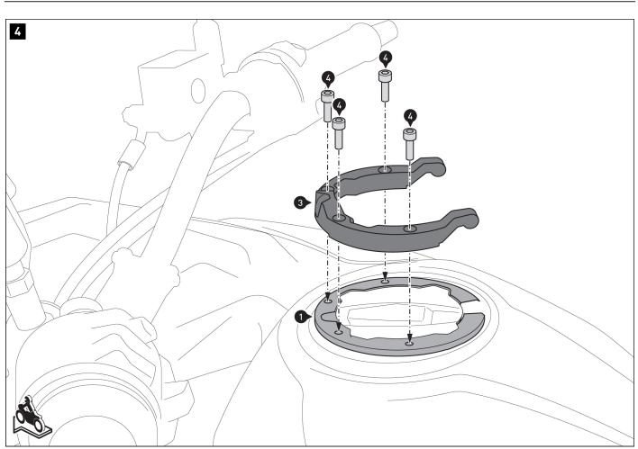
Screw the tank ring (3) onto the tank ring adaptor (1).
