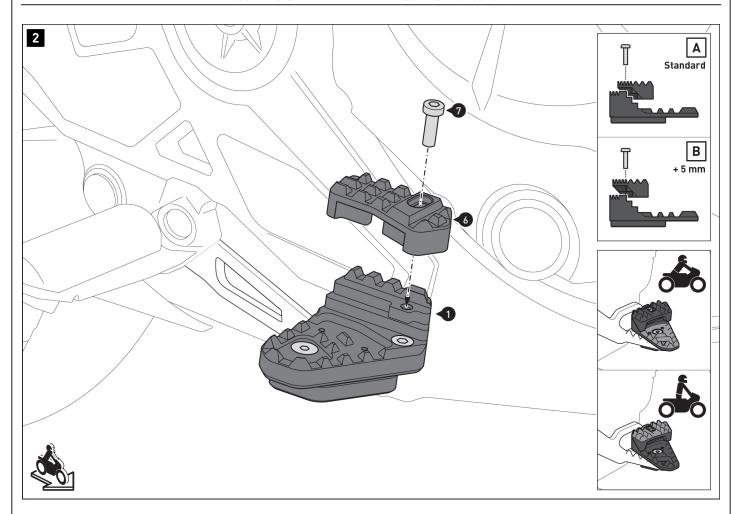
Screw the elevation (6) onto the extension (1) in position [A] (standard) or [B] (+ 5 mm).
