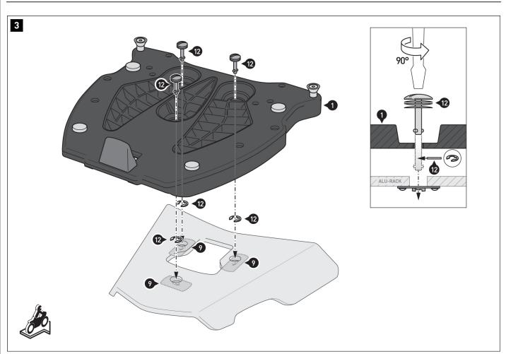
Insert the quick-release fasteners (12) into the openings on the adapter plate (1). Secure the quick-release fasteners (12) with the enclosed circlips as shown in the detailed drawing. Then place the adapter plate (1) onto the ALU-RACK; a quarter turn of the quick release fasteners (12) attaches the adapter plate (1) to the ALU-RACK.
